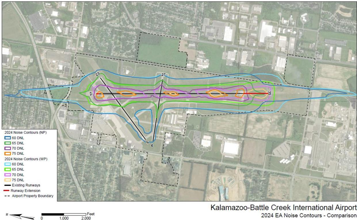
**Figure 9.0: 2029 AZO Noise Contour Comparisons – Existing and Extended Runways**
