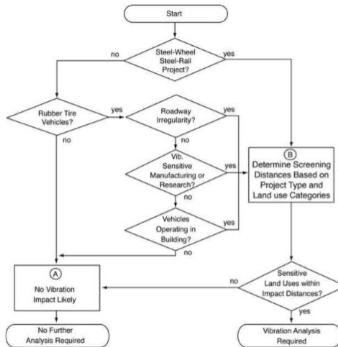
**Figure 6-3 Flow Chart of Vibration Screening Process**
